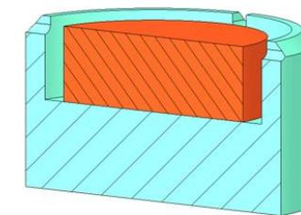
Cross-sectional view of the cup containing the fuel disk (modification of existing design)
