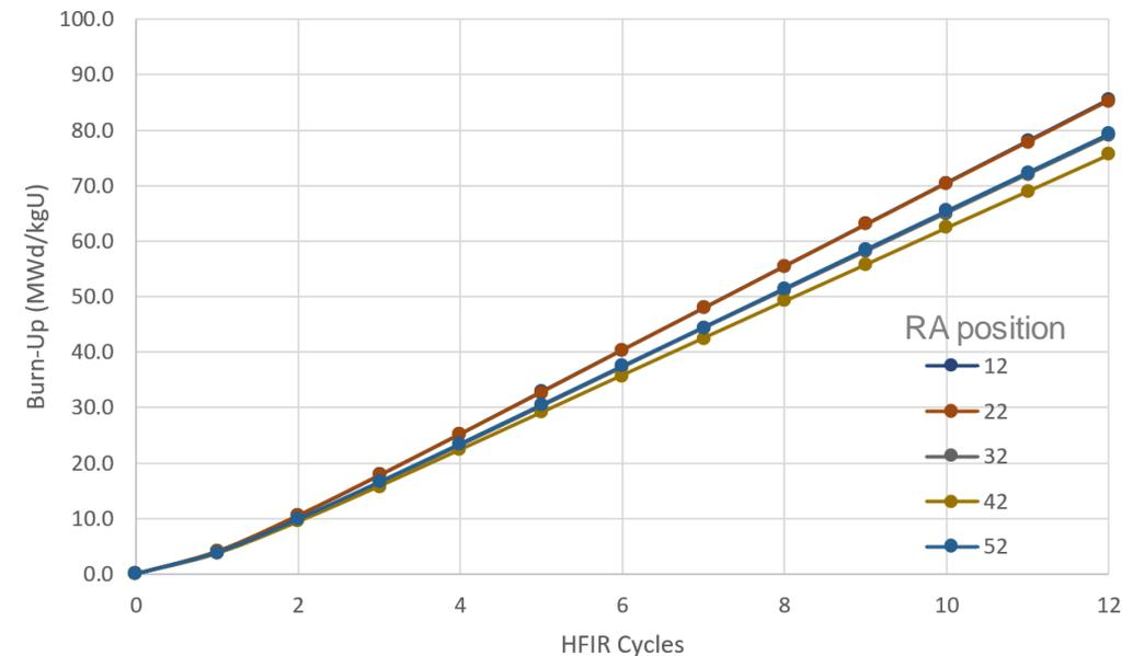
Average fuel specimen burnup for 5 targets positions as a function of the number of HFIR cycles
