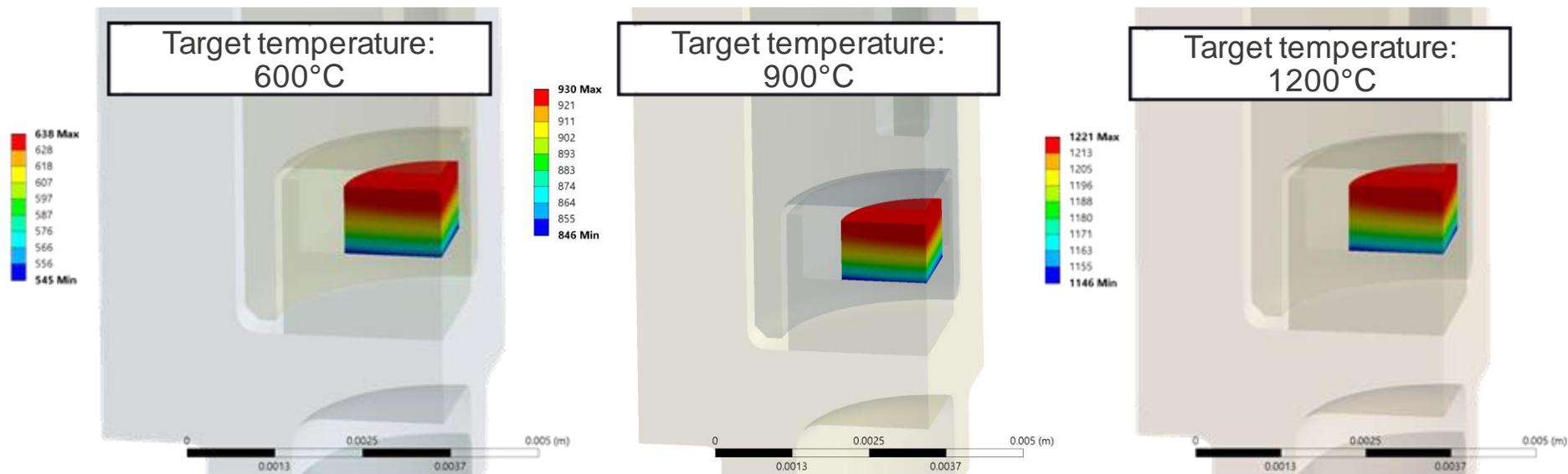
Temperature contours of the fuel specimens for the 3 target temperatures
