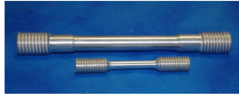
ASTM standard tensile bars: yield strength, modulus, % elongation
