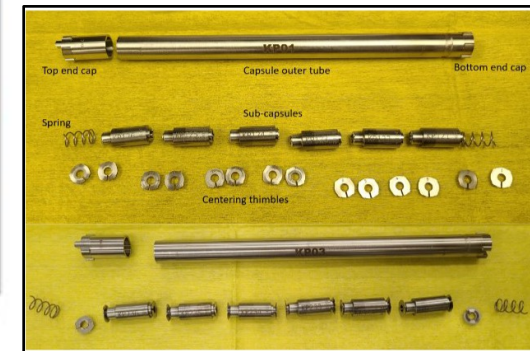
Irradiation Targets with Sub-Capsules
