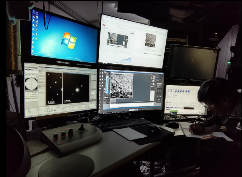
In-situ TEM irradiation of a FeCrAl alloy in MIBL-(MC) 2 Results courtesy of K. Sun and H. Li (UM)
