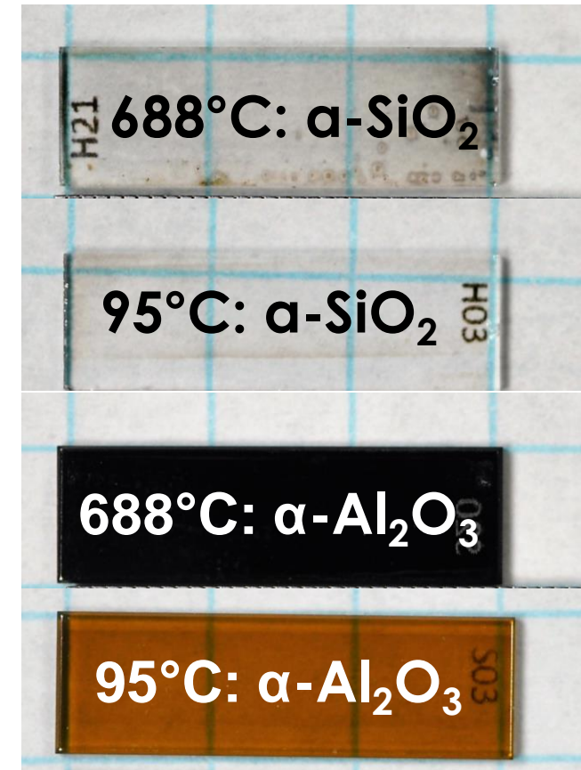
Post-irradiation pictures of \alpha -SiO 2 and \alpha -Al 2 O 3 specimens
