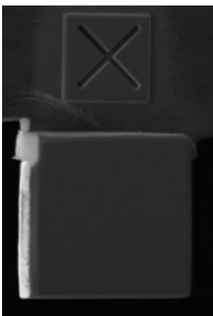
FIB Milling – SEM View
