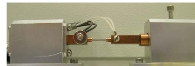
Spring loaded resistance measurement fixture. The SiC monitor is held in place between the two copper electrodes.
