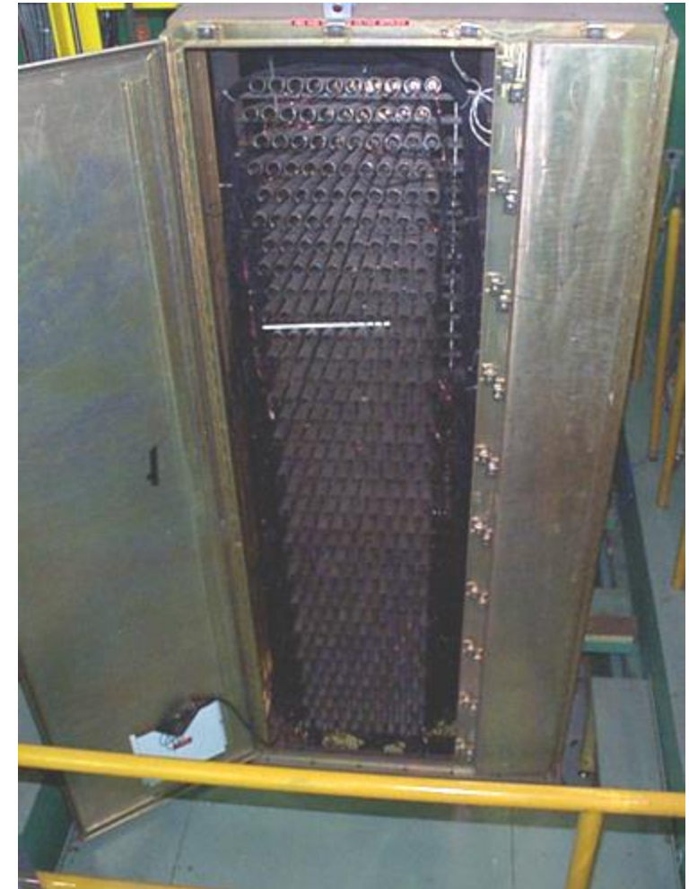
View of the Hodoscope system from the rear with the detector panel open
