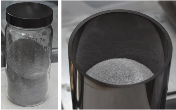
Figure 4. Uranium metal powder, ammonium chloride, and lithium chloride – potassium chloride blend before (left) and after (right) loading in glassy carbon crucible.
