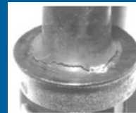
Stress corrosion cracking
