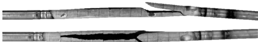
Cladding failure and dispersed fuel inventory for high burnup fuel, NEA-6847
