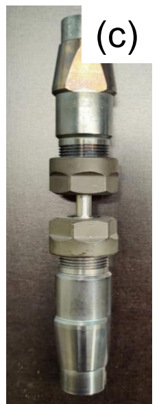
FIG. 12 Metal Plugs for Testing Tubular Specimens, Proper Location of Plugs in Specimen and of Specimen in Heads of Testing Machine
