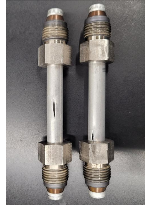
Tested specimens, featuring Swagelok fittings
