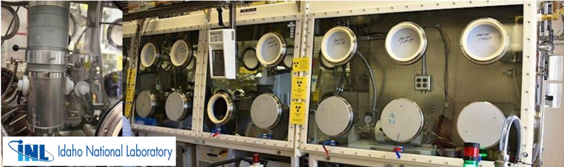
Simultaneous thermal analyzer, dilatometer, LFA, DSC inside of the fresh fuels glovebox (FFG)
