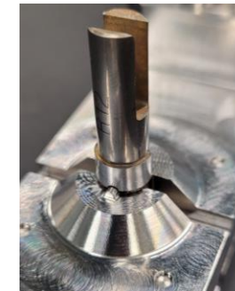
Mandrels in loading orientation with ring specimen installed.
