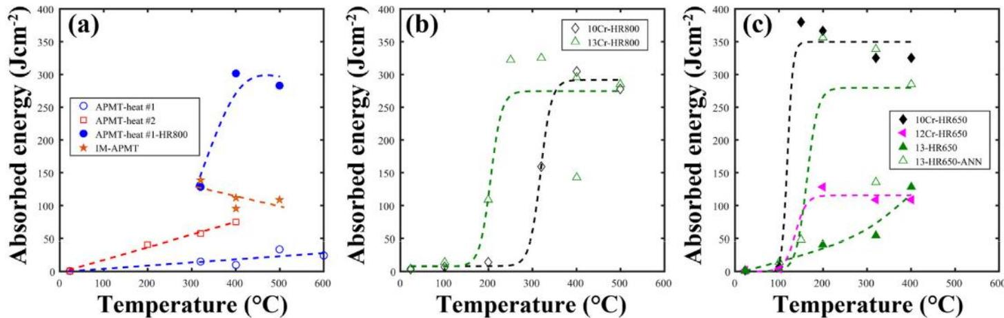
**Fig. 8.** Impact absorbed energy in the temperature range from RT to 600 °C for (a) commercial APMT alloys and their variations; (b) wrought FeCrAl alloys hot-rolled at 800 °C; and (c) wrought FeCrAl alloys hot-rolled at 650 °C.
