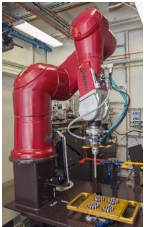
Robot for high-throughput sample changing
